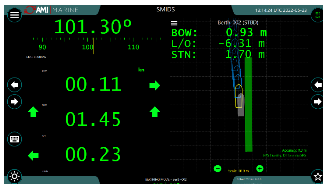
SMIDS Berthing Information Page (Fore and Aft Speed, Bow/Stern Sideways Movement Speeds, Gyro Heading and Vessel Berthing Assist)
