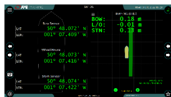
SMIDS Berth and Lat/Lon (Vessel Berthing Assist and individual Bow/Stern Latitude and Longitude)
