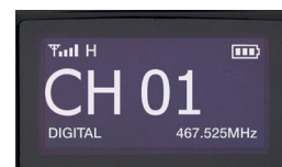
Informative display shows the channel number and the frequency
